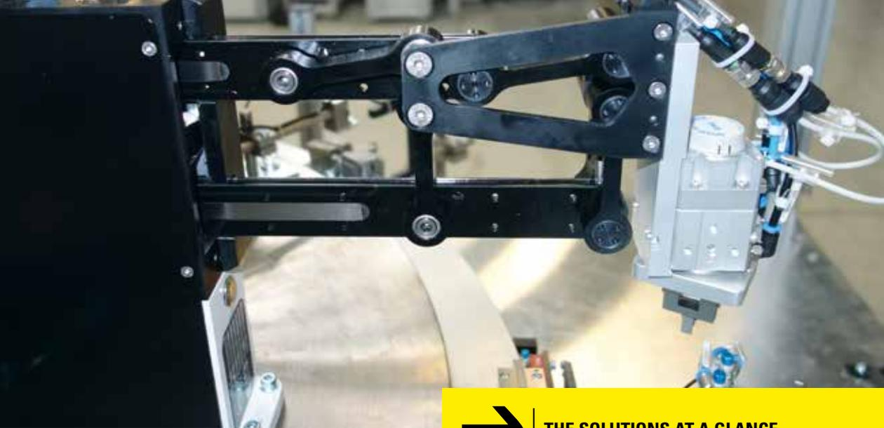
**The kinematic unit of the HP 70 enables a vertical stroke of 70 millimetres. The maximum horizontal stroke is 325 millimetres. Thanks to the programmability of the axes, every point within this operating range can be reached on freely selectable tracks.**
