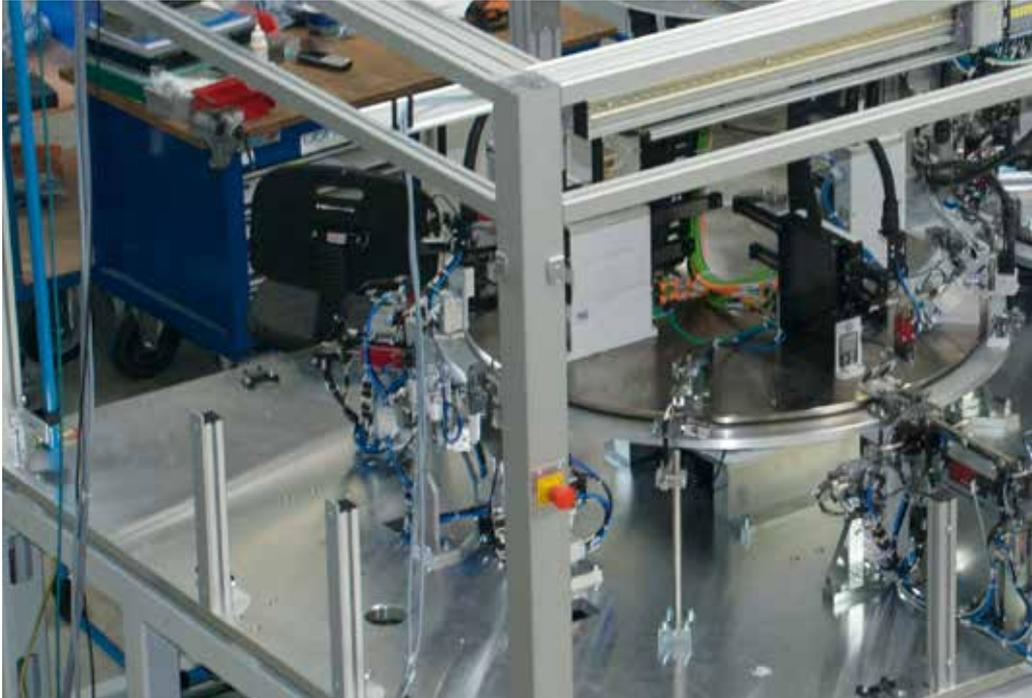
**Automated assembly system for electromechanical sensors: 3 rotary indexing tables and 11 direct-drive pick & place units from WEISS. From a single source and perfectly matched to one another. The combination offers positioning accuracy of 0.02 millimetres.**
